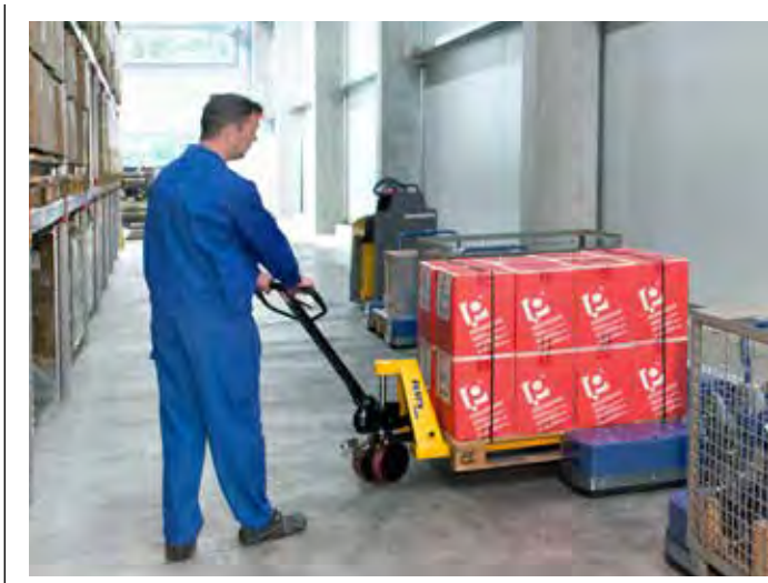
(Ont)laden d.m.v. handpallettruck
